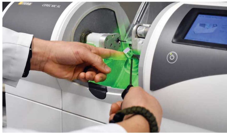
Kroll uses a milling machine to grind a crown (left). He inserts a block of dental ceramic (above), and 3D coordinates are used to create the crown.
