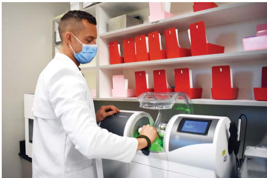
Kroll uses a milling machine to grind a crown (left). He inserts a block of dental ceramic (above), and 3D coordinates are used to create the crown.
